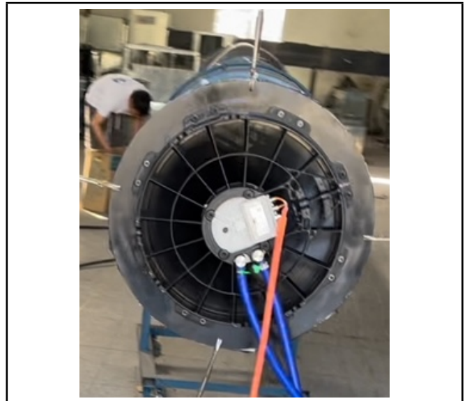
Figure 11. Efficiency test in a wind tunnel.
