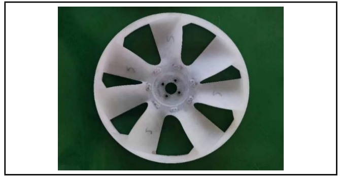
Figure 15. Test sample of the optimal leading triangle and uneven arrangement design.
