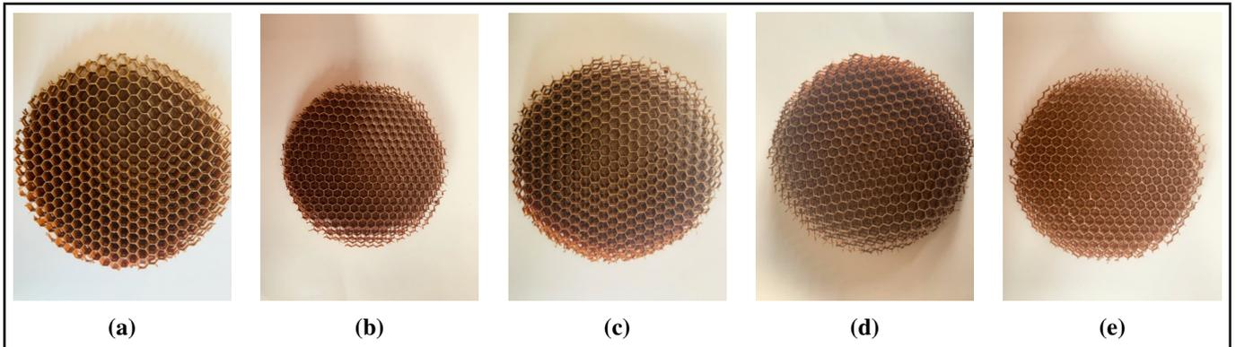
**Figure 13.** The first set of experiments (changing the number of dislocation layers of honeycomb): (a) No. 1, dislocation zero layer; (b) No. 2, dislocation two layers; (c) No. 3, dislocation three layers; (d) No. 4, dislocation four layers; (e) No. 5, dislocation five layers.
