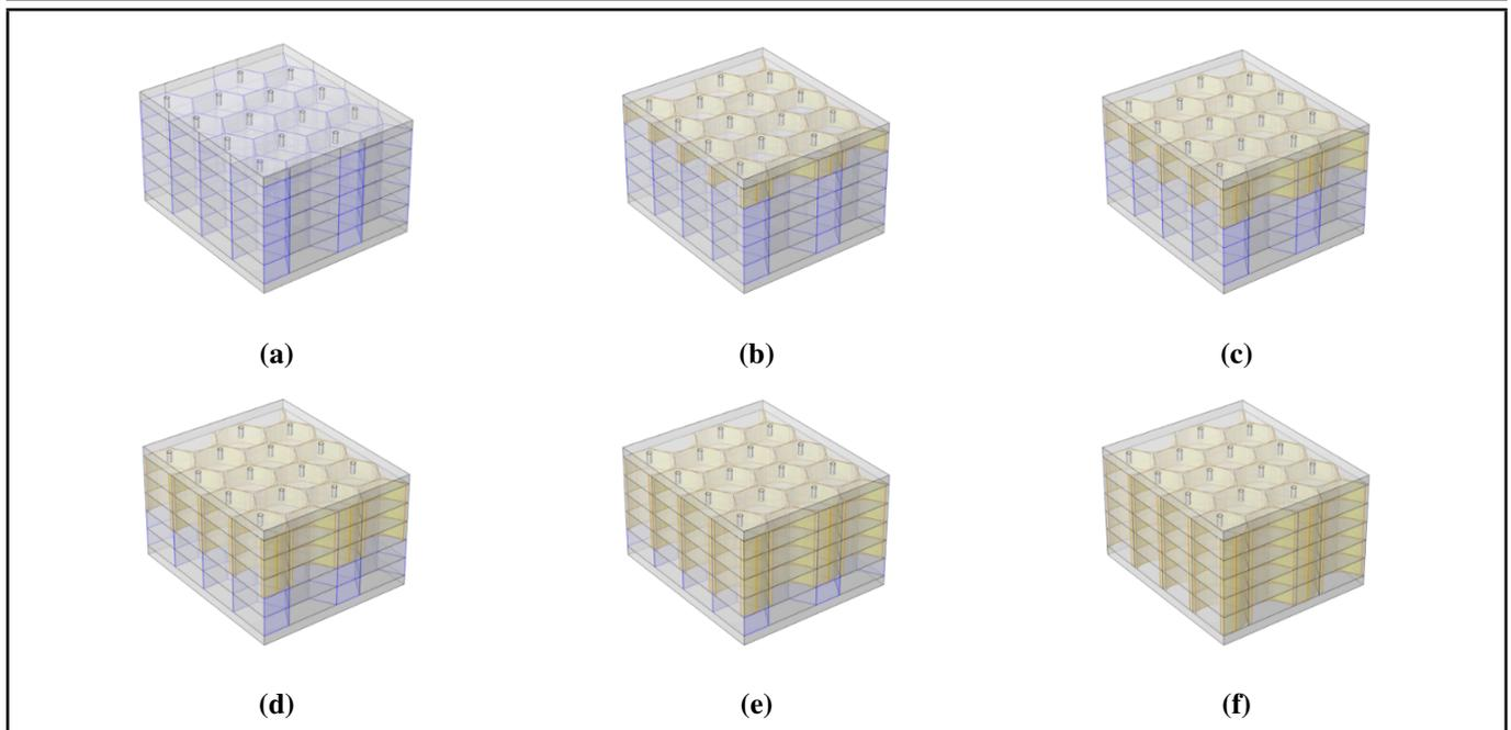
**Figure 3.** Honeycomb core layers with different diatom mud coating layers: (a) zero layer; (b) one layer; (c) two layers; (d) three layers; (e) four layers; (f) five layers.
