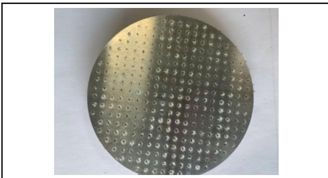
Figure 7. Microperforated plate for experiment.
