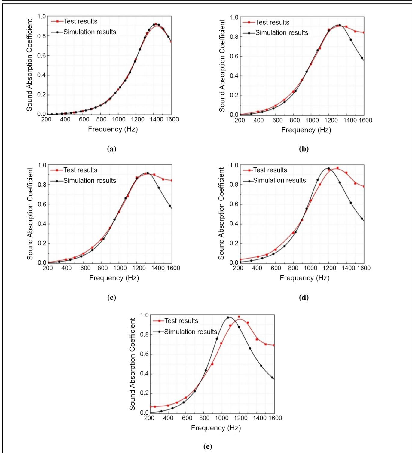
**Figure 18.** Fitting of test results and simulation results: (a) zero layer; (b) two layers; (c) three layers; (d) four layers; (e) five layers.
