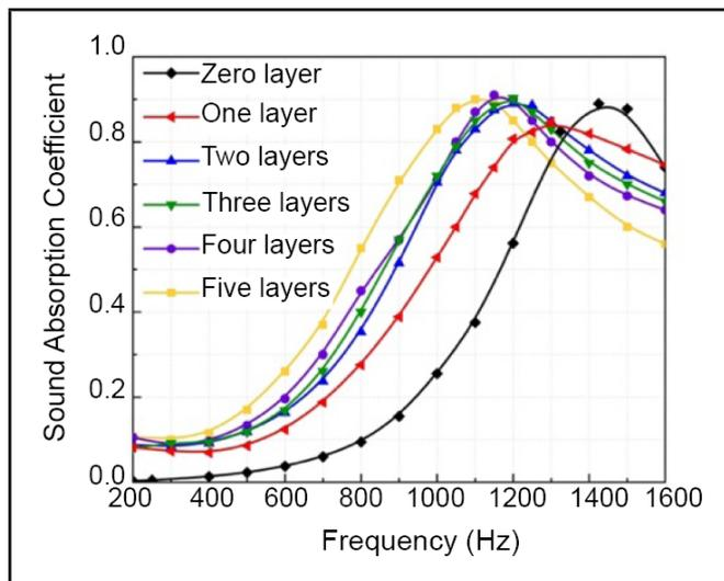
**Figure 19.** The effect of the number of coating layers on the sound absorption performance.
