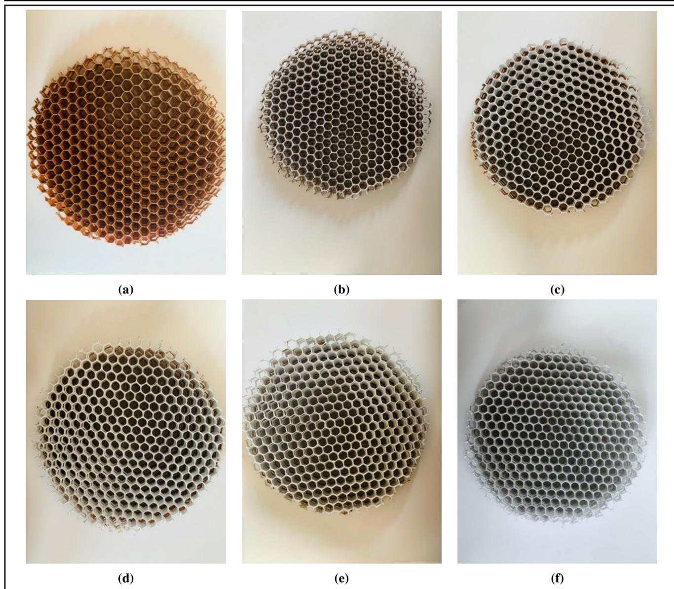
**Figure 14.** The second group of experiments (changing the number of aligned honeycomb diatom mud coatings): (a) No. 6, zero-layer coating; (b) No. 7, one-layer coating; (c) No. 8, two-layer coating; (d) No. 9, three-layer coating; (e) No. 10, four-layer coating; (f) No. 11, five-layer coating.
