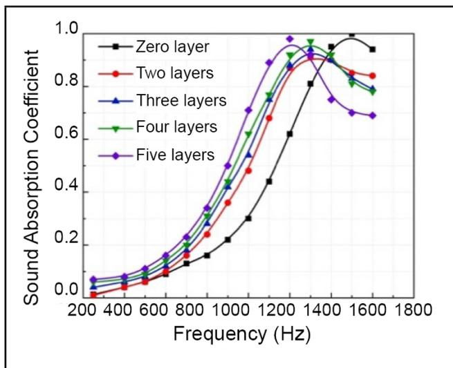
**Figure 16.** The effect of the number of dislocation layers on the sound absorption performance.
