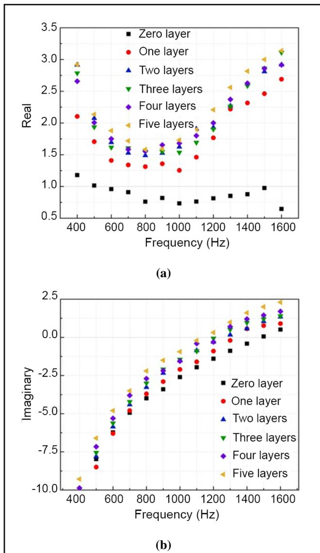
**Figure 20.** The effect of the number of coating layers on the acoustic impedance: (a) acoustic resistance; (b) acoustic impedance.
