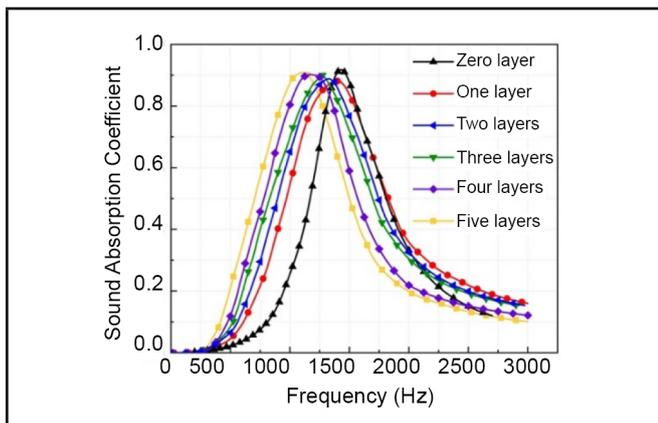
**Figure 4.** Simulation results of the effect of the number of coating layers on the sound absorption coefficient.
