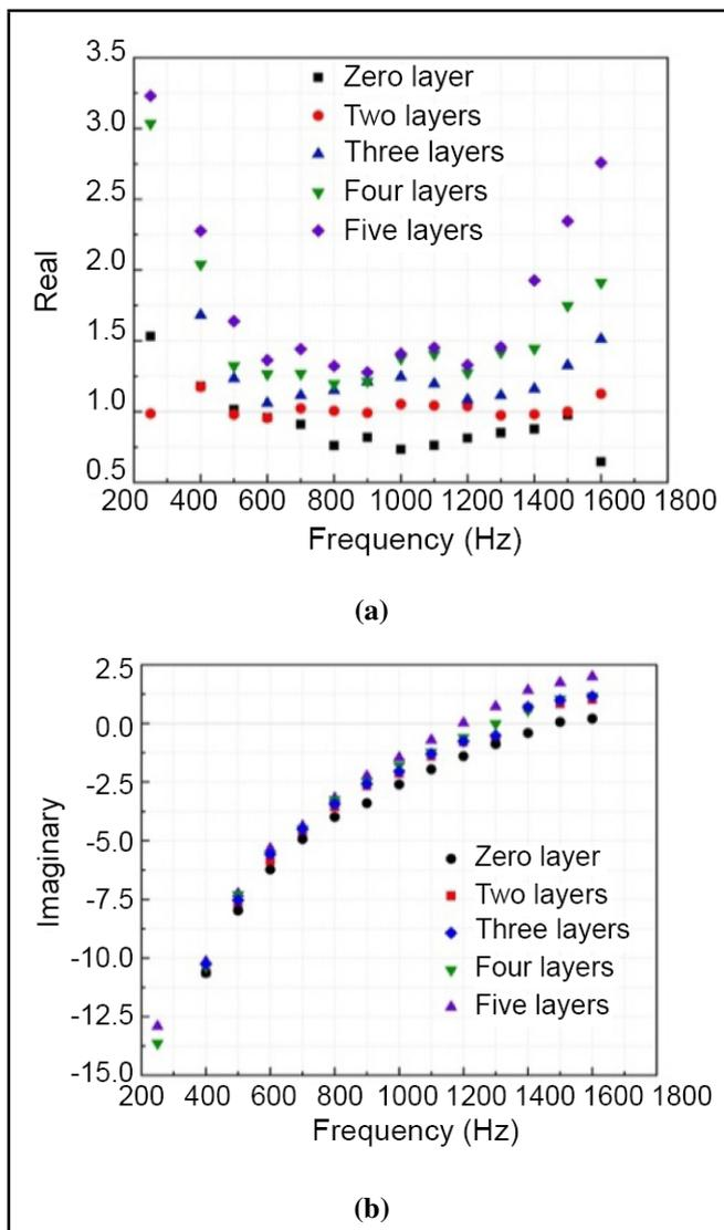
**Figure 17.** The effect of the number of dislocation layers on the acoustic impedance: (a) acoustic resistance; (b) acoustic impedance.
