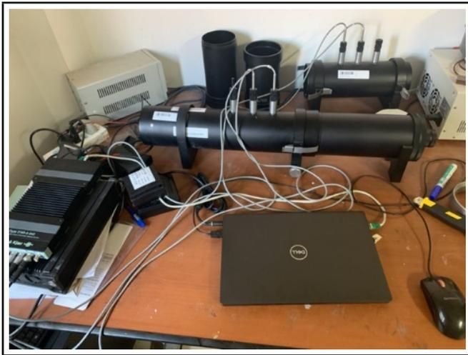
Figure 5. Impedance tube test device.
