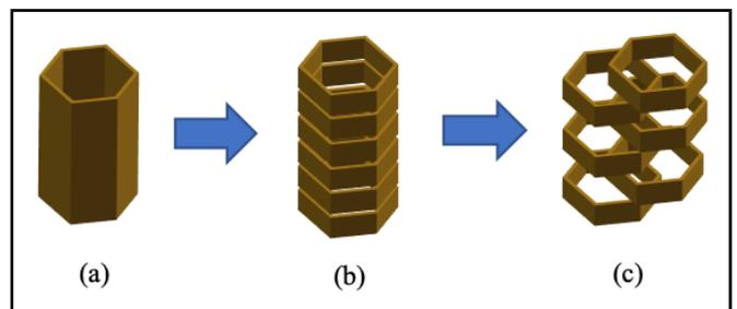
Figure 10. Traditional aligned honeycomb and misaligned stacked honeycomb.
