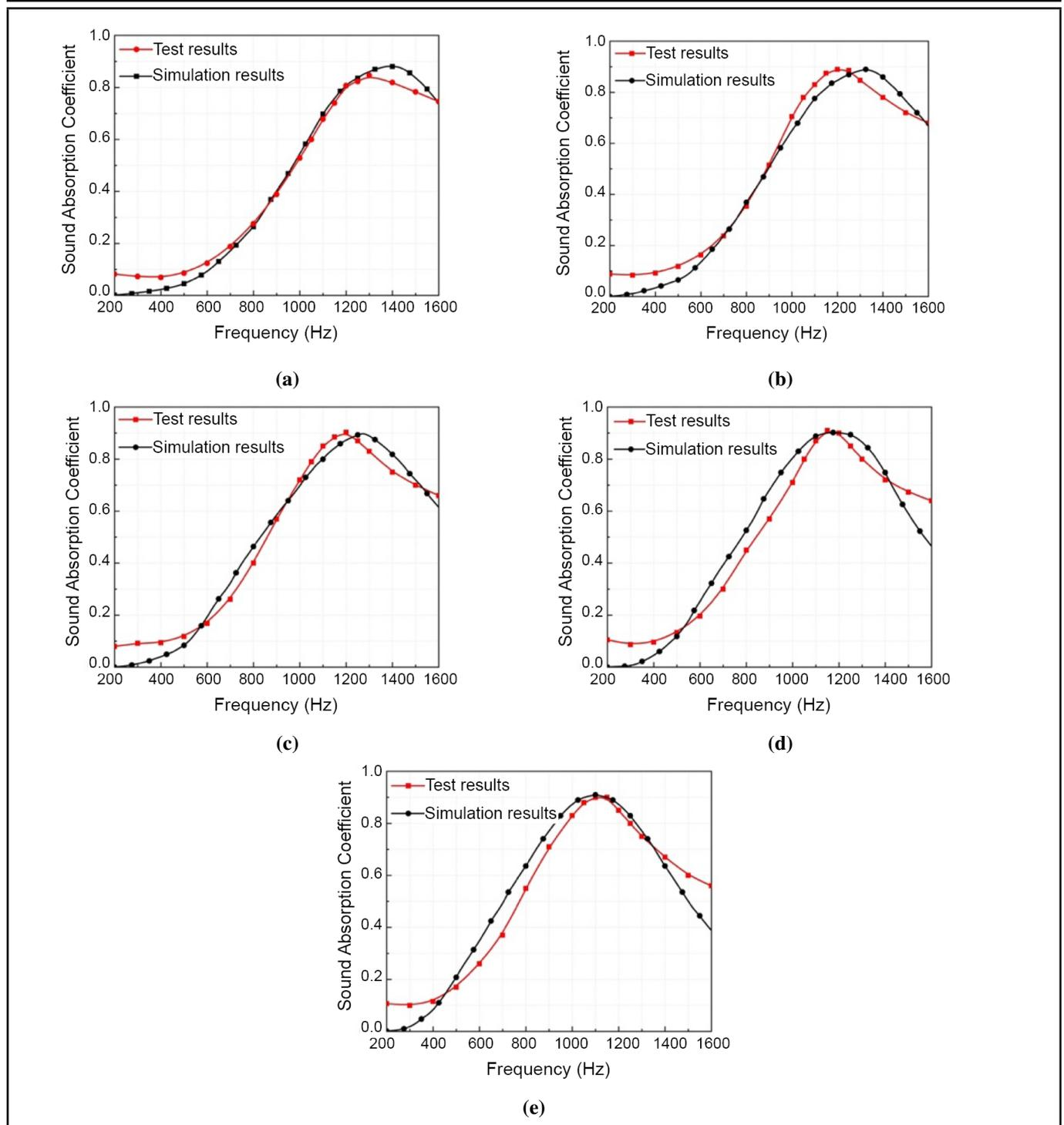
**Figure 21.** Fitting of test results and simulation results: (a) one layer; (b) two layers; (c) three layers; (d) four layers; (e) five layers.
