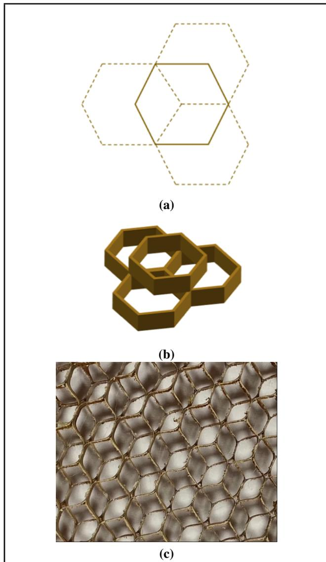
**Figure 11.** Schematic diagram of dislocation arrangement: (a) plan view; (b) three-dimensional view; (c) physical view.
