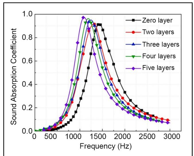
**Figure 2.** Simulation results of the effect of the number of dislocation layers on the sound absorption coefficient.
