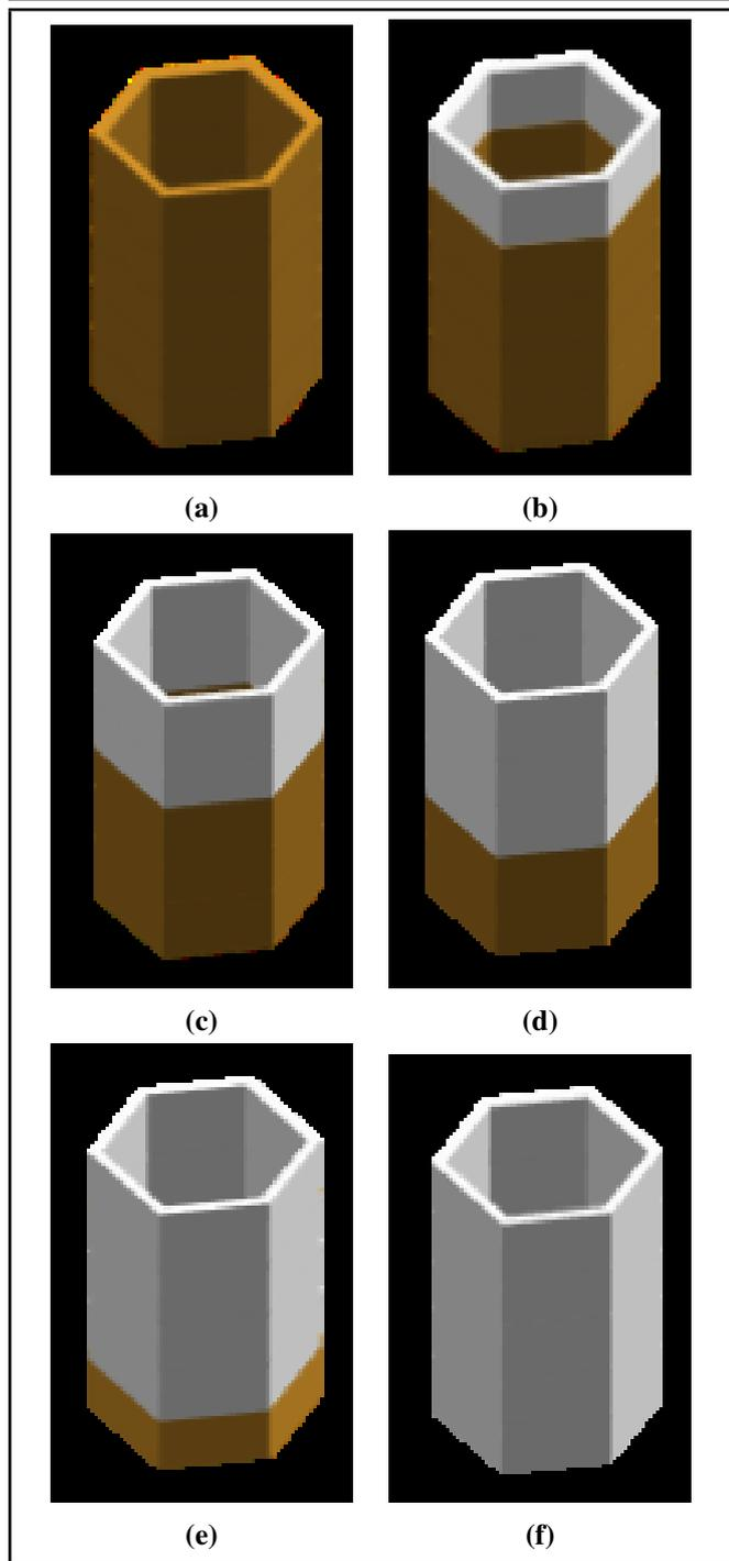
**Figure 15.** Schematic diagram of honeycomb cells with different coating layers: (a) zero layer; (b) one layer; (c) two layers; (d) three layers; (e) four layers; (f) five layers.
