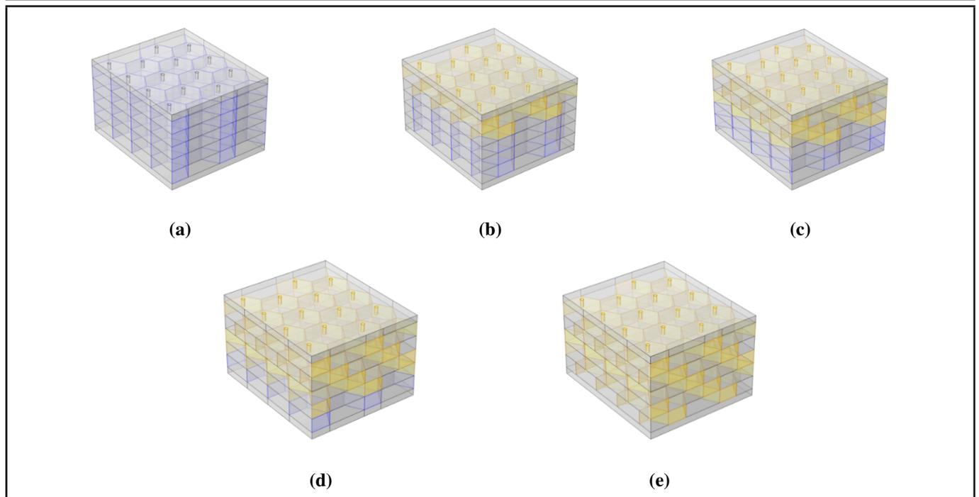
**Figure 1.** Honeycomb core layers with different dislocation layers: (a) zero layer; (b) two layers; (c) three layers; (d) four layers; (e) five layers.
