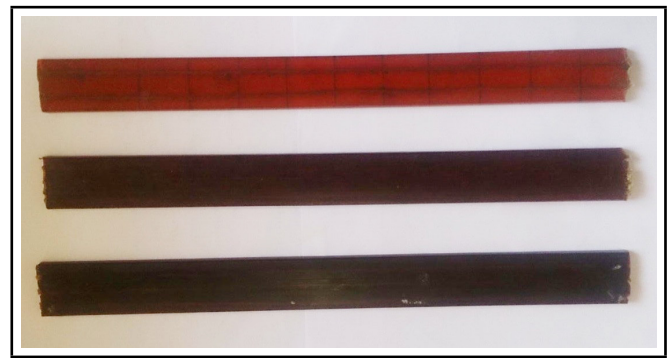
Figure 2. Composite samples for vibration with no fibre discontinuity.
