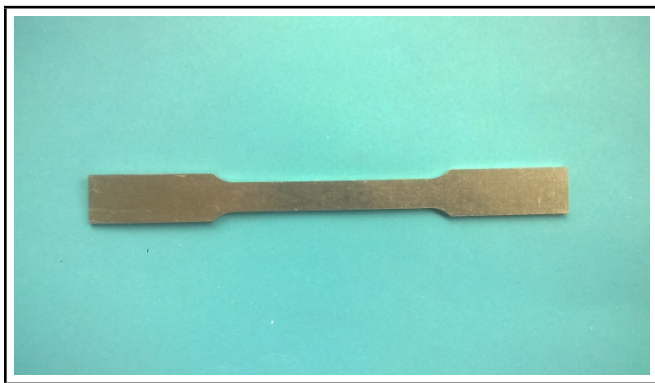
Figure 1. AA 2219 tensile test specimen.
