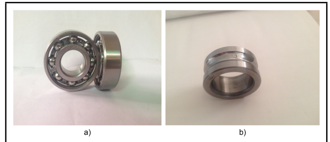
Figure 4. a) 6204 Bearings at normal state. b) 6204 Bearing with inner ring pitting.
