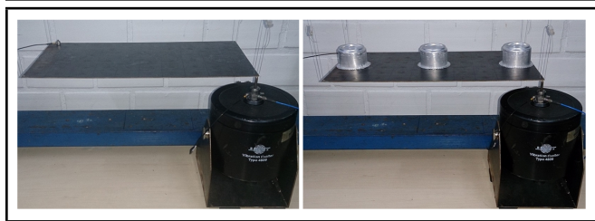
Figure 8. Steel plate with free boundary conditions. The vibration exciter was located at a corner of the plate and the accelerometer at the elements of the uniformly discretized plate. Left: Plate without dampers. Right: Plate with 3 EPDs. Dimensions are shown in Fig. 7.
