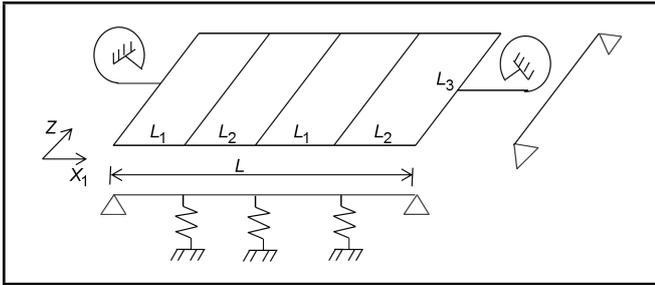
Figure 2. An unfolded plate representation of a simply supported rectangular duct.
