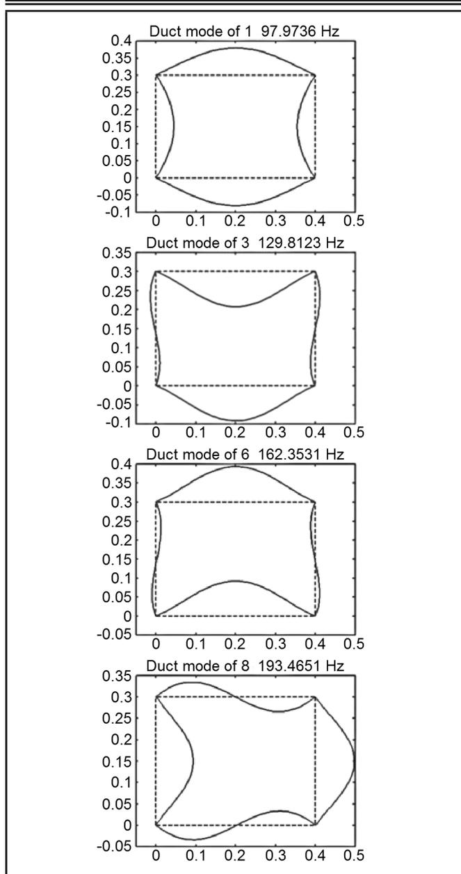
Figure 3. Mode shapes for the 1<sup>st</sup>, 3<sup>rd</sup>, 6<sup>th</sup>, and 8<sup>th</sup> natural frequencies of a rectangular duct with S-S boundary conditions.
