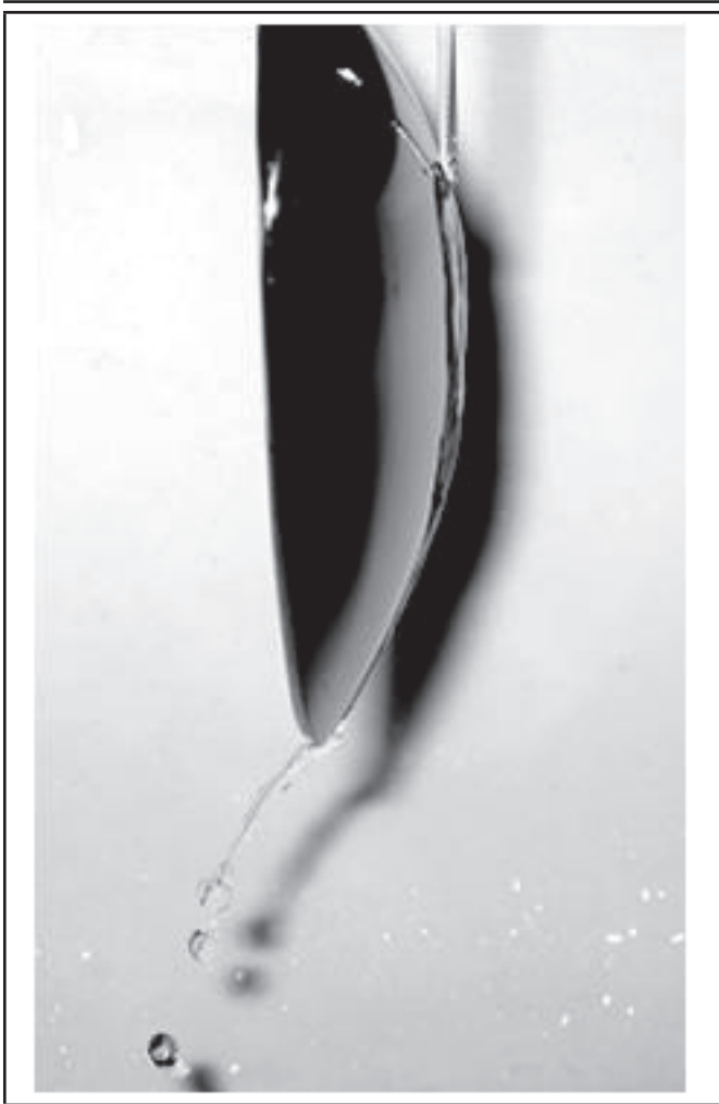
Figure 2. The Teapot effect (Image by Axda0002 at en.wikipedia [CC-BY-SA-2.5 ( www.creativecommons.org/licenses/by-sa/2.5 )], via Wikimedia Commons).
