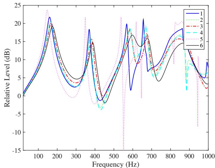
**Figure 5.** Simulated FRF at the **Receiver  $R_3$**  for different geometry configurations. Blue and solid line = configuration 1, green and dotted line = configuration 2, red and dashdot line = configuration 3, cyan and dashed line = configuration 4, magenta and dotted faint line = configuration 5 and black and solid faint line = configuration 6.
