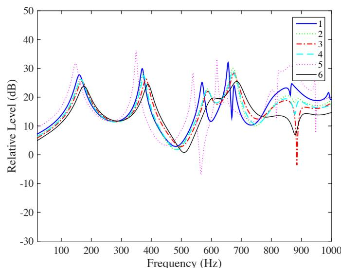
**Figure 4.** Simulated FRF at the **Receiver  $R_2$**  for different geometry configurations. Blue and solid line = configuration 1, green and dotted line = configuration 2, red and dashdot line = configuration 3, cyan and dashed line = configuration 4, magenta and dotted faint line = configuration 5 and black and solid faint line = configuration 6.
