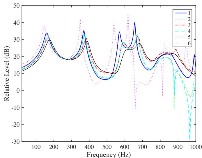
**Figure 3.** Simulated FRF at the **Receiver  $R_1$**  for different geometry configurations. Blue and solid line = configuration 1, green and dotted line = configuration 2, red and dashdot line = configuration 3, cyan and dashed line = configuration 4, magenta and dotted faint line = configuration 5 and black and solid faint line = configuration 6.
