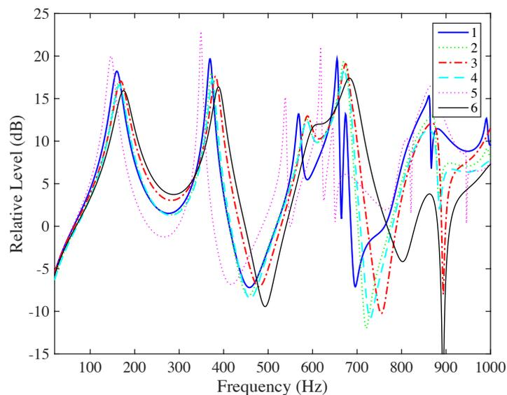
**Figure 6.** Simulated FRF at the **Receiver  $R_4$**  for different geometry configurations. Blue and solid line = configuration 1, green and dotted line = configuration 2, red and dashdot line = configuration 3, cyan and dashed line = configuration 4, magenta and dotted faint line = configuration 5 and black and solid faint line = configuration 6.
