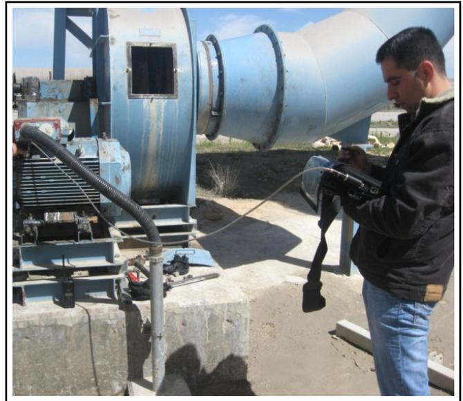
Figure 5. Measurement of vibrations of Bearing A.
