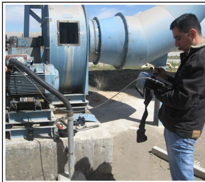
Figure 5. Measurement of vibrations of Bearing A.
