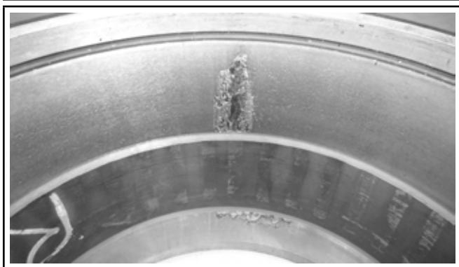
Figure 3. Cup raceway spall that developed naturally in service and was pulled from the field.
